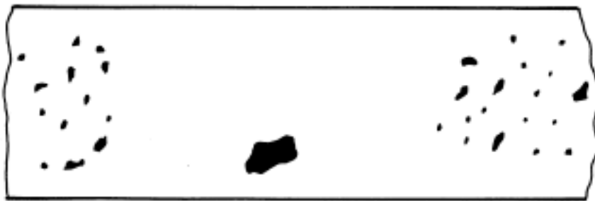
ASSORTED POROSITY Typical concentration of size permitted in any 150 mm length of weld
