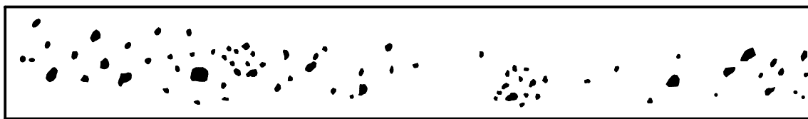
ASSORTED POROSITY Typical concentration and size permitted in any 150 mm length of weld
